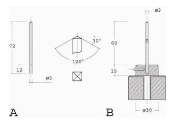
Figure A.1. High speed dynamometer for test of cloth resistance to perforation
