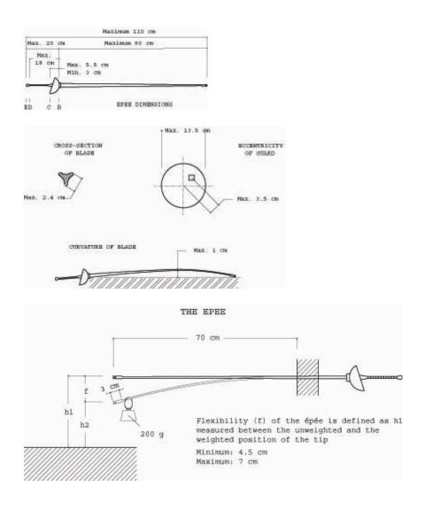
Figure 9. Epee dimensions and flexibility
